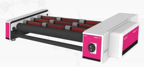
**Usage** - mixing of blood samples and viscous substances
